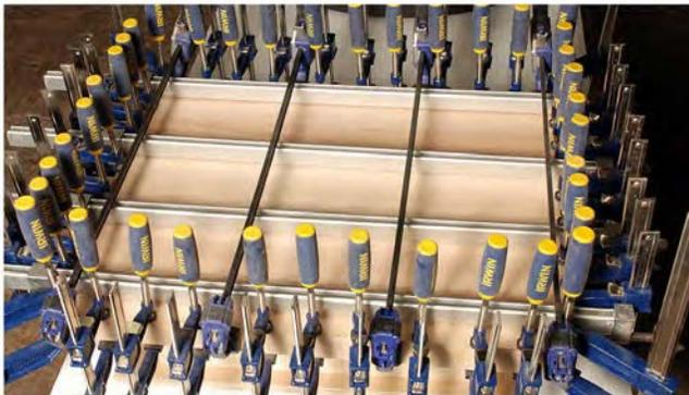
To assemble our tables, every piece is excessively clamped to ensure the glue joint will never fail. The consistent pressure keeps the skirt and top snugly joined and uniform in strength. You can never use too many clamps.
