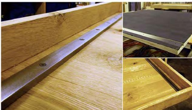
Our superior construction includes laminating solid steel stock to the underside of the table top and filling it in with formaldehyde free Baltic birch plywood. The steel is screwed in four inch intervals and bonded to the wood with superior poly adhesive. This extra step in construction prevents cupping and bowing, a common problem with lesser quality tables.
