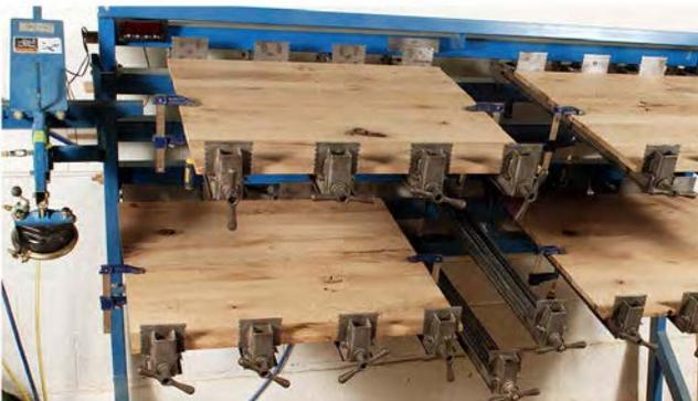
Assembly of our tables begins at the clamp rack. Once the wood has been sourced and selected, we glue and flatten our boards using our JLT Industrial Clamp Racks with a Pneumatic flattener. Tightly clamped, our boards come out flat, strong, and with a sturdy glue-up to ensure long lasting tables.
