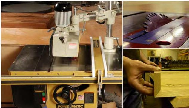
Our unique, mitre-fold construction creates a thickness and stability seldom seen in any table. To assemble our mitre-fold, we feed our planed wood through our Powermatic table saw for a perfect 45 degree cut, every time. This ensures our tables will withstand years and years of continuous use.
