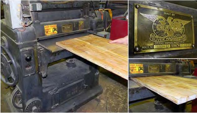
When the top surface is assembled, it is then planed to produce a uniform surface on the top and bottom faces. Sometimes vintage tools make the best tools. We use a 1952 Oliver Planer to create the flattest, cleanest, and smoothest piece of wood imaginable.
